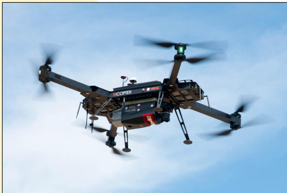
APX-20 and nadir RGB camera fully integrated
