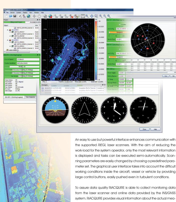
To assure data quality RiACQUIRE is able to collect monitoring data from the laser scanner and online data provided by the INS/GNSS system. RiACQUIRE provides visual information about the actual measurements from the INS/GNSS system to easily check the plausibility of the results. A continuous recording of system status, INS/GNSS attitude and position, and all the interactions of the operator with RiACQUIRE,
