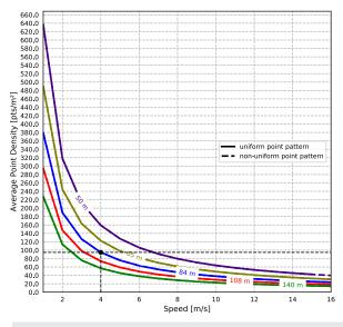
Example: miniVUX-3UAV at 200,000 pulses/second, speed = 4 m/s, range to target =  $\sim$  85 m, resulting point density  $\sim$  95 pts/m<sup>2</sup>
