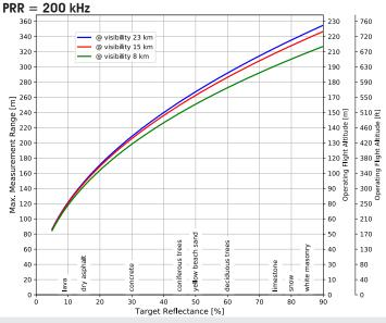
Operating Flight Altitude AGL given for the following conditions: FOV of +/-45°, target size ≥ laser footprint, average ambient brightness
