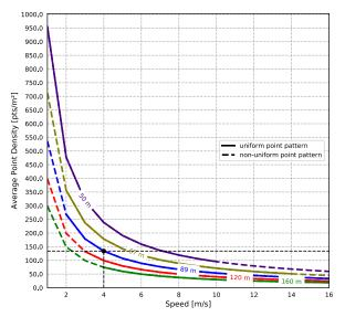
Example: miniVUX-3UAV at 300,000 pulses/second, speed = 4 m/s, range to target =  $\sim$  90 m, resulting point density  $\sim$  135 pts/m²
