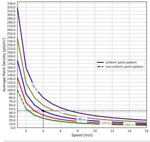
Example: miniVUX-3UAV at 100,000 pulses/second, speed = 4 m/s, range to target =  $\sim$  90 m, resulting point density  $\sim$  45 pts/m<sup>2</sup>
