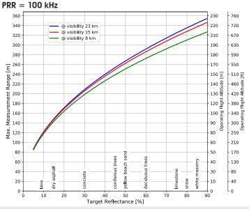
Operating Flight Altitude AGL given for the following conditions: FOV of  $+/-45^\circ$ , target size  $\geq$  laser footprint, average ambient brightness
