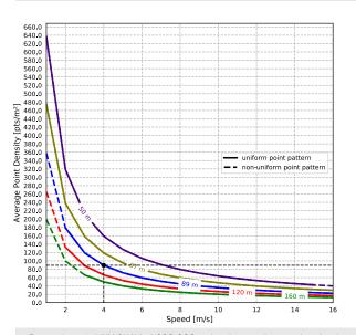
Example: miniVUX-3UAV at 200,000 pulses/second, speed = 4 m/s, range to target =  $\sim$  90 m, resulting point density  $\sim$  90 pts/m<sup>2</sup>
