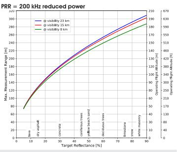
Operating Flight Altitude AGL given for the following conditions: FOV of +/-45 $^{\circ}$ , target size  $\geq$  laser footprint, overcast sky, ambient brightness 10klx
