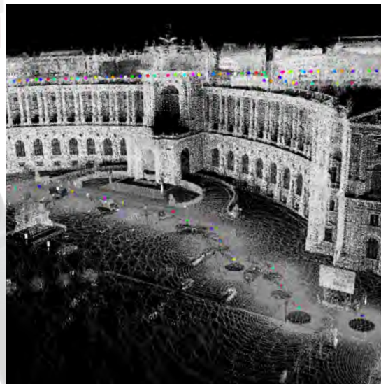
scan data detail, reflectance-scaled
