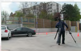
move the scanner to the next scan position
