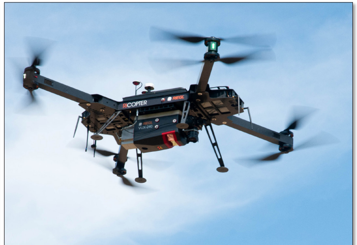
RICOPTER with RIEGL VUX-240 LiDAR Sensor, APX-20 UAV and nadir RGB camera fully integrated
