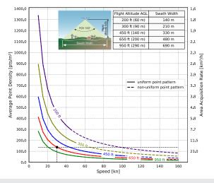
Example: VUX-160 $^{23}$  at 1,200,000 pulses/sec, laser power level 100% altitude 650 ft AGL, speed 30 kn, resulting point density  $\sim$  137 pts/m $^2$
