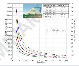
Example: VUX-16023 at 2,400,000 pulses/sec, laser power level 100% altitude 500 ft AGL, speed 30 kn, resulting point density  $\sim$  356 pts/m²
