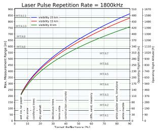
Operating Flight Altitude AGL given for the following conditions: FOV 100°, ambiguity resolved by multiple-time-around (MTA) processing, average ambient brightness, target size  $\geq$  laser footprint, roll angle  $<\pm5$  deg
