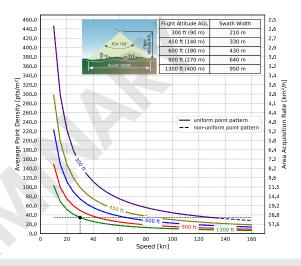
Example: VUX- $160^{23}$  at 600,000 pulses/sec, laser power level 100% altitude 1,300 ft AGL, speed 30 kn, resulting point density  $\sim 34$  pts/m<sup>2</sup>
