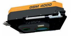
RIEGL VQ-840-G (with external IMU) installed on GSM-4000 stabilized platform to be used in a helicopter or fixed-wing aircraft
