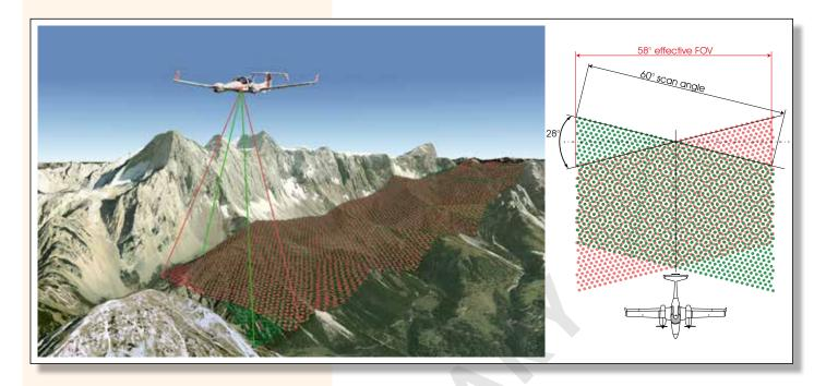
Each channel delivers straight parallel scan lines. The scan lines of the two channels are tilted against each other by 28 degrees providing an optimum distribution of the measurements on the ground invariant to changes in terrain height.
