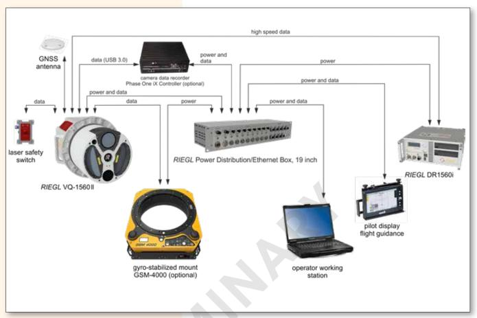
A minimum number of system components and external cabling is required for an easy and quick installation in aircrafts.
