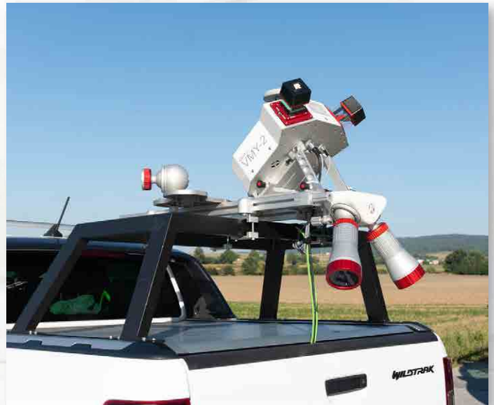
NADIR orientation of the RIEGL cameras with pavement mount
