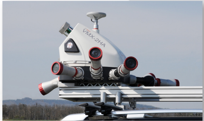
VMX-2HA equipped with 7 ball-joint directional RIEGL cameras
