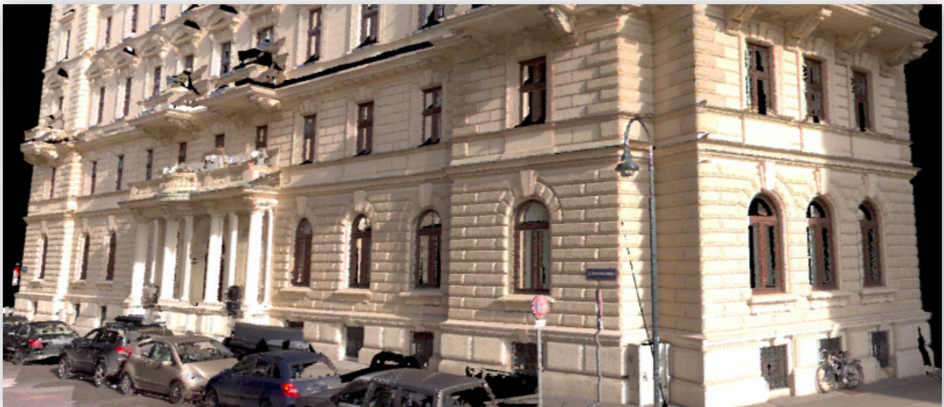
colored point cloud: image data captured by FLIR Ladybug® 5+
