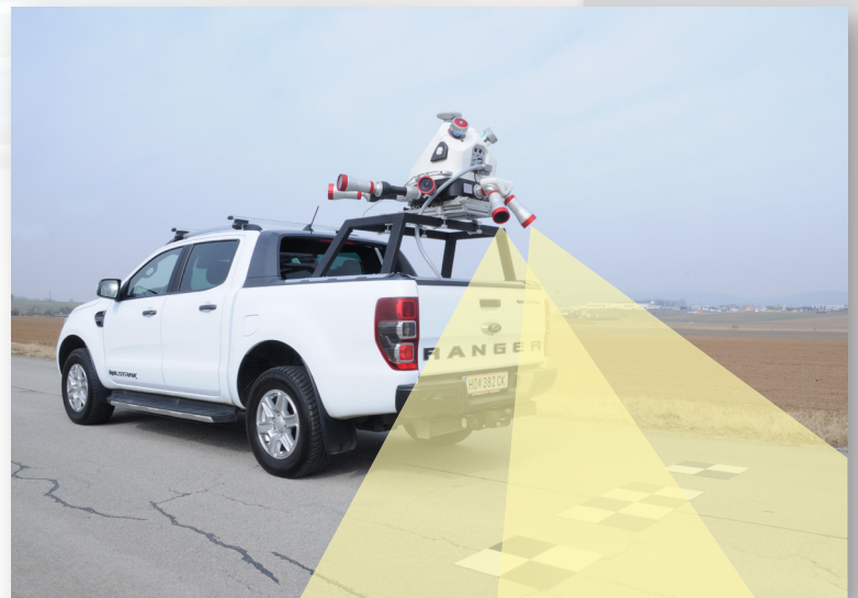
VMX-2HA equipped with 6 ball-joint directional RIEGL cameras, two ball-joint pavement cameras with NADIR orientation and a Ladybug 5+
