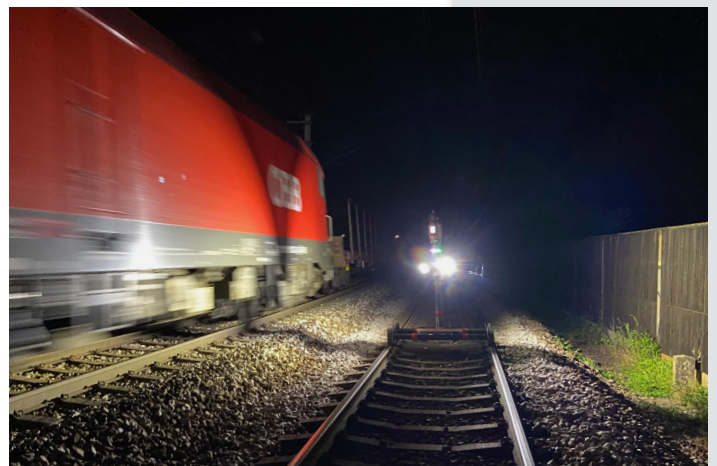
optional lighting system with 4 LED lights
