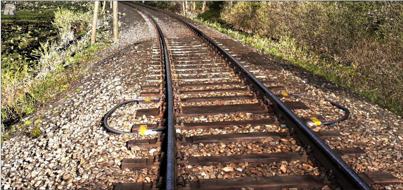
true-colored point cloud acquired in RISCAN PRO
