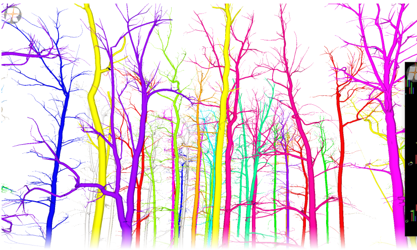
Segmented trees colored according to a unique tree ID: Each tree is georeferenced. A so-called pipe model is created for each tree – this is used to perform a highly accurate volume calculation. Branches can also be separated from trunks.
