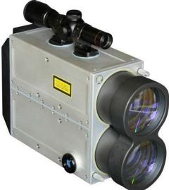
The *RIEGL* LD05-A80 is a multi-purpose laser distance meter based on precise time-of-flight laser range measurement. It uses state-of-the-art **digital signal processing** enabling precise distance measurement for complex multi-target situations even under bad visibility conditions. Digitizing the echo signal and subsequent analyzing allows multitarget distance measurements. Up to 5 target distances can be detected and provided for each laser shot.
