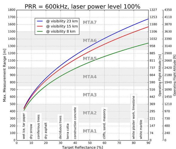
**Example:** VQ-480 II at 600,000 pulses/sec, laser power level 100%
