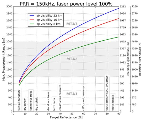
**Example:** VQ-480 II at 150,000 pulses/sec, laser power level 100%
