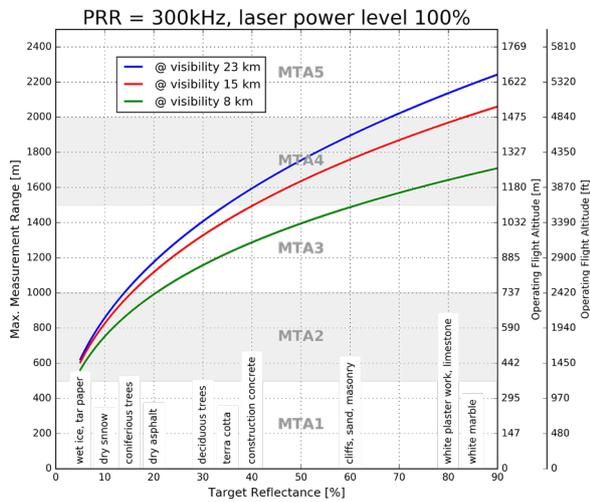
**Example:** VQ-480 II at 300,000 pulses/sec, laser power level 100%
