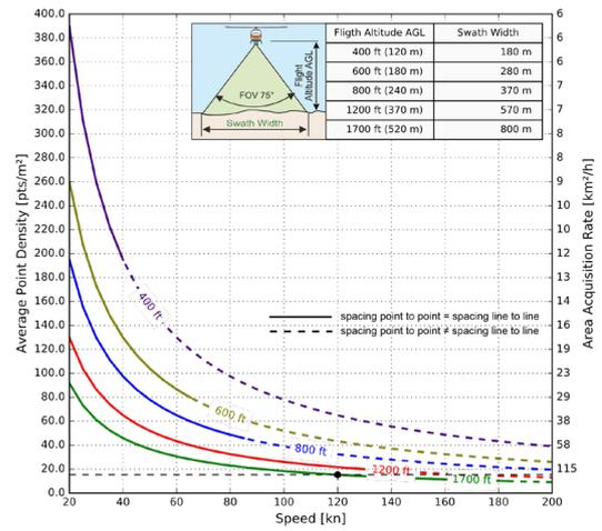
**Example:** VQ-480 II at 1,200,000 pulses/sec, laser power level 100%
