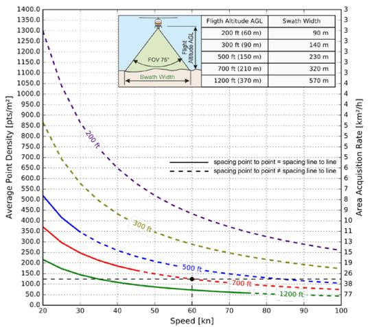
**Example:** VQ-480 II at 2,000,000 pulses/sec, laser power level 100%
