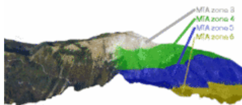
Automatic Multiple Time Around processing (pulses in the air)
