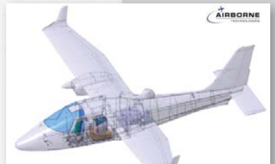
RIEGL LMS-Q1560 installed on GSM-3000 stabilized platform in the fixed-wing aircraft TECNAM MMA
