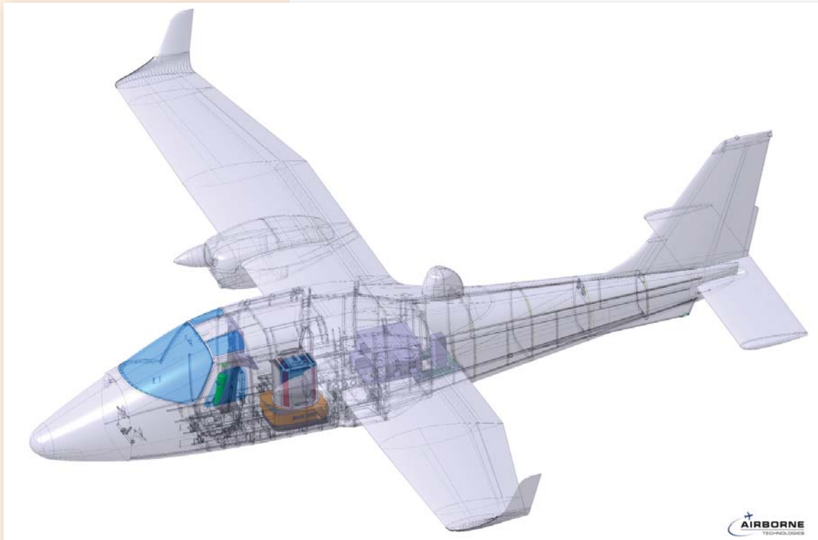
RIEGL LMS-Q1560 installed on GSM-3000 stabilized platform in the fixed-wing aircraft TECNAM MMA
