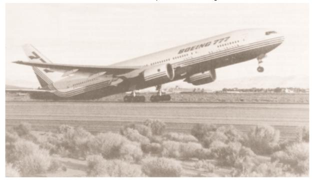
BOEING NEWS OCT. 7 / 1994: The first Boeing 777 strikes its tail on a runway at Edwards Air Force Base, Calif., as it performs one of many precertification tests. This test, called a velocity minimum unstick, or VMU, is used to determine the airplane's minimum takeoff speed. The test requires the airplane's protected tail to come in contact with the runway prior to takeoff. Boeing incorporates data from the test into flight manuals used by the airlines.
