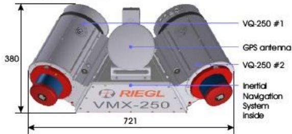
VMX-250-MH Measuring Head
